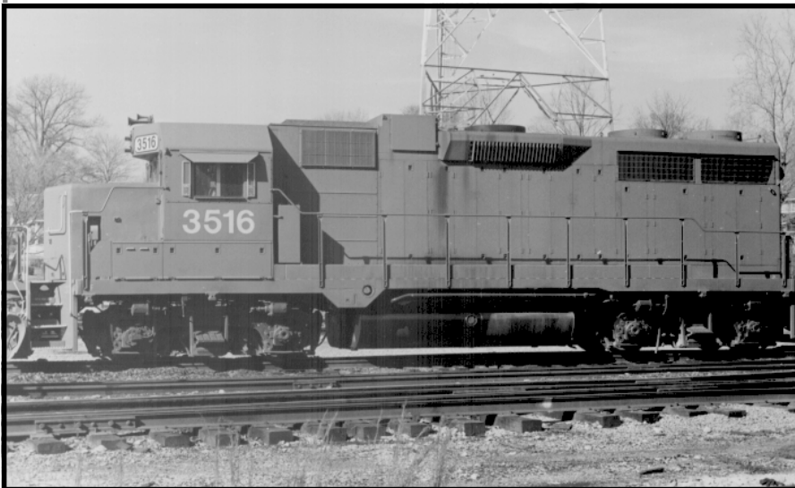
ExICG ExxGM&O GP35 repowered with Caterpillar Diesel engine by VMV. The unit rides on Blomberg trucks rather than the original Alco trucks. This project was not repeated and the unit was sold. Photo taken at Central City, KY on February 19, 1990. Photo by Chuck Hinrichs
